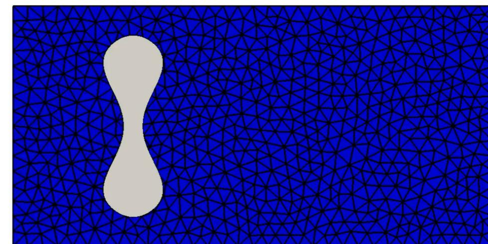
Development of numerical methods that use **general polygonal and polyhedral mesh elements** (es. **Virtual Element Method**, **Polygonal Discontinuous Galerkin**, HDG, Weak Galerkin, Mimetic Finite Differences, Hybrid High Order, etc...).
