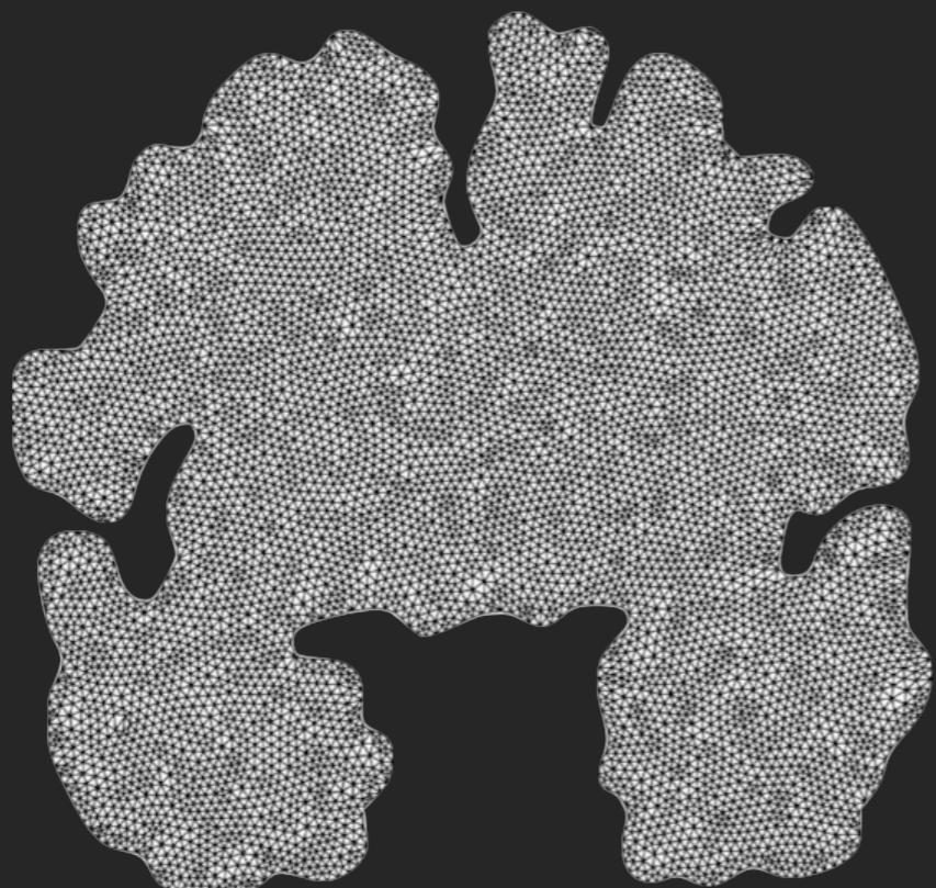
Merging neighboring mesh elements to obtain a coarser grid.
