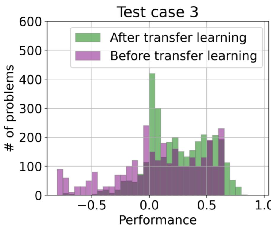
Improving efficiency of algebraic multigrid methods through artificial neural networks: choosing the strong threshold parameter  $\theta$  as the one the ANN predicts to give the best performance.
