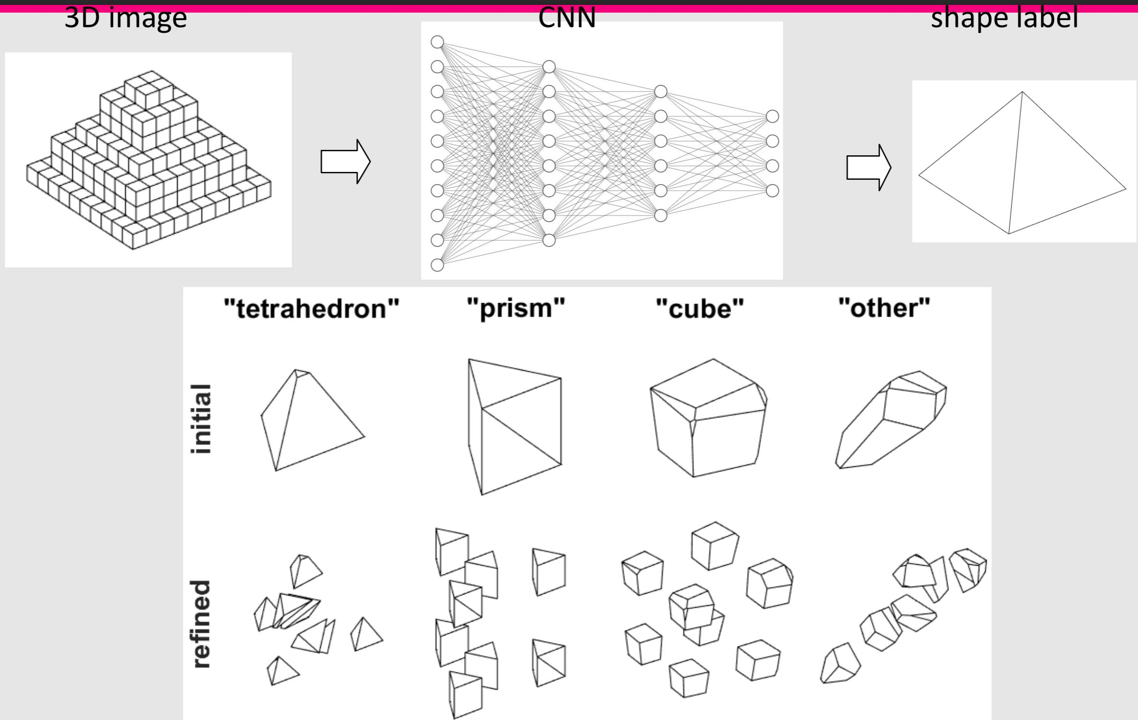
The CNN classifies the 3D image of the input polyhedron according to its shape, in order to apply suitable refinement strategies. Elements in class "other" are refined using the k-means strategy.
