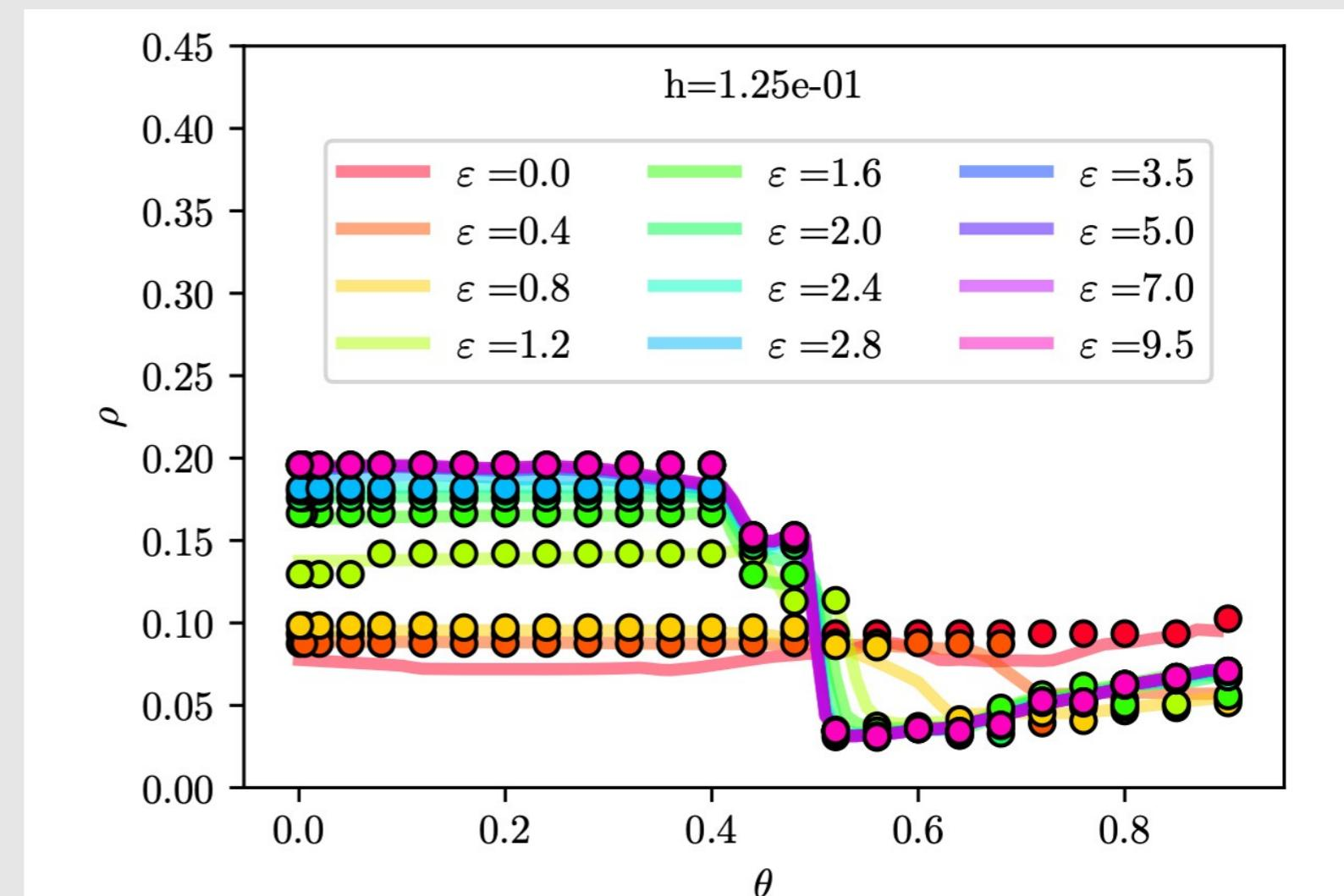
Improving efficiency of algebraic multigrid methods through artificial neural networks: choosing the strong threshold parameter  $\theta$  as the one the ANN predicts to give the best performance (  $\approx 30\%$  gain)
