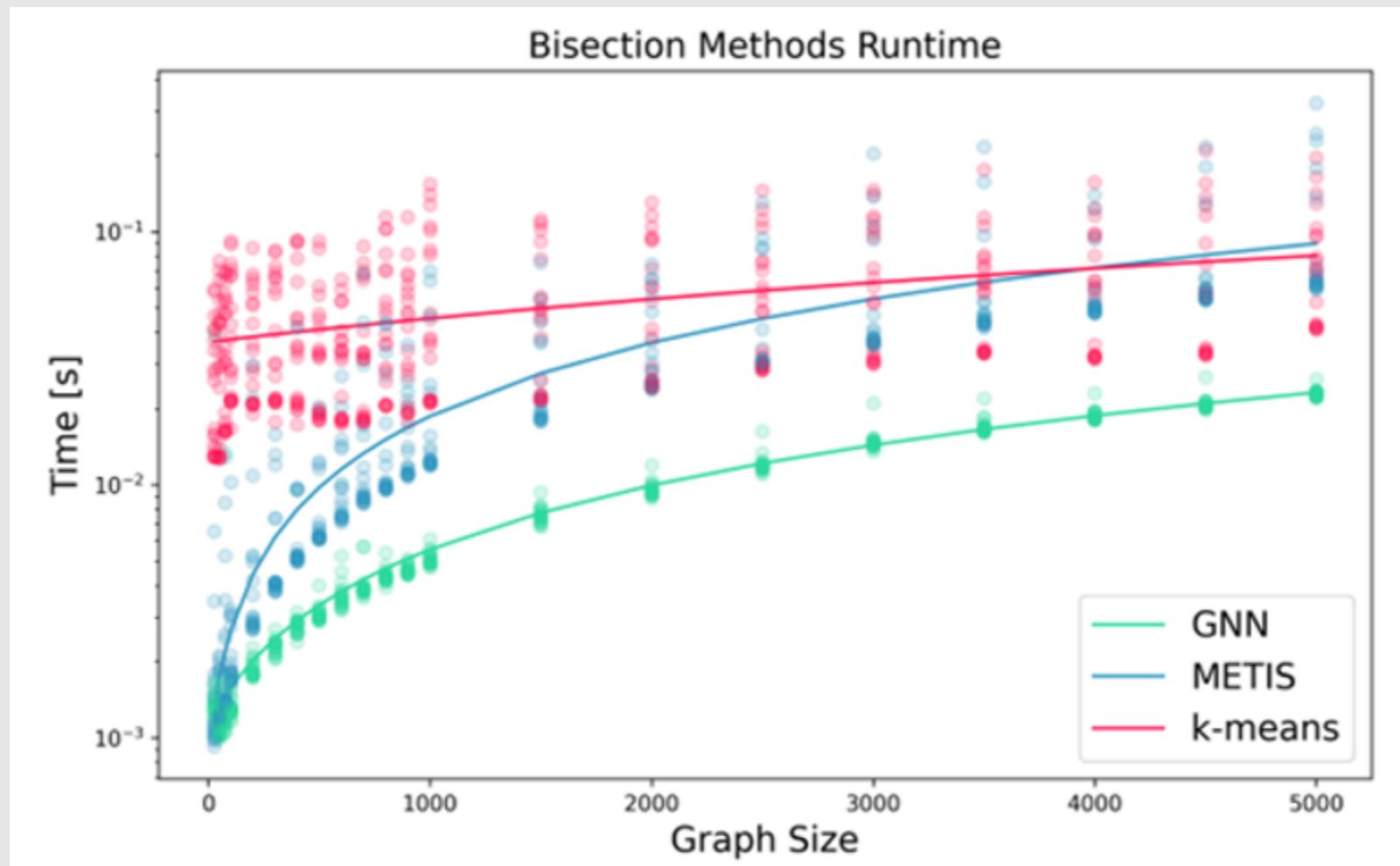
Runtime performance for different graph bisection models (METIS, k-means, GNN) as a function of the number of nodes in the connectivity graph of Voronoi meshes. The y-axis is in logarithmic scale
