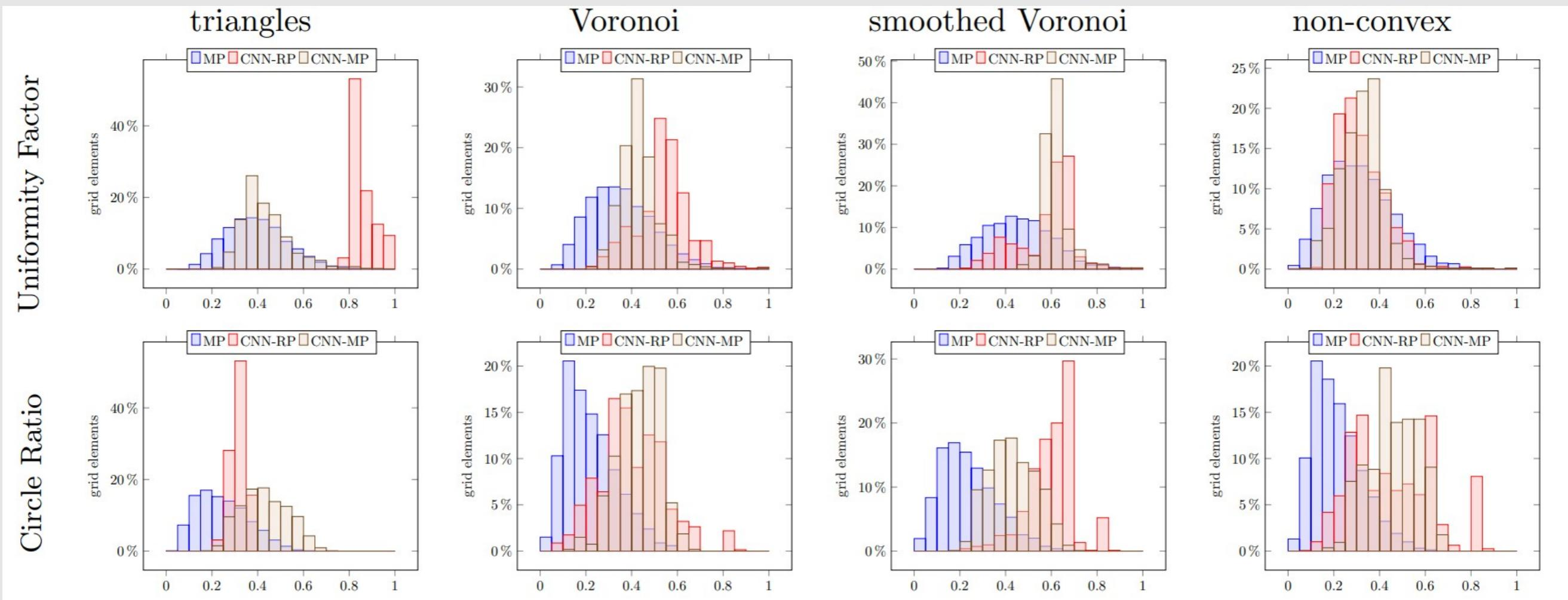
$$\text{Uniformity Factor} = \frac{\text{element size}}{\text{mesh size}}$$
